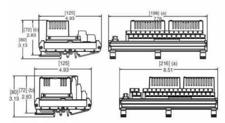
(a) Overall width — for determining DIN rail loading, (b) Height above DIN rail (add to DIN rail height for total).
